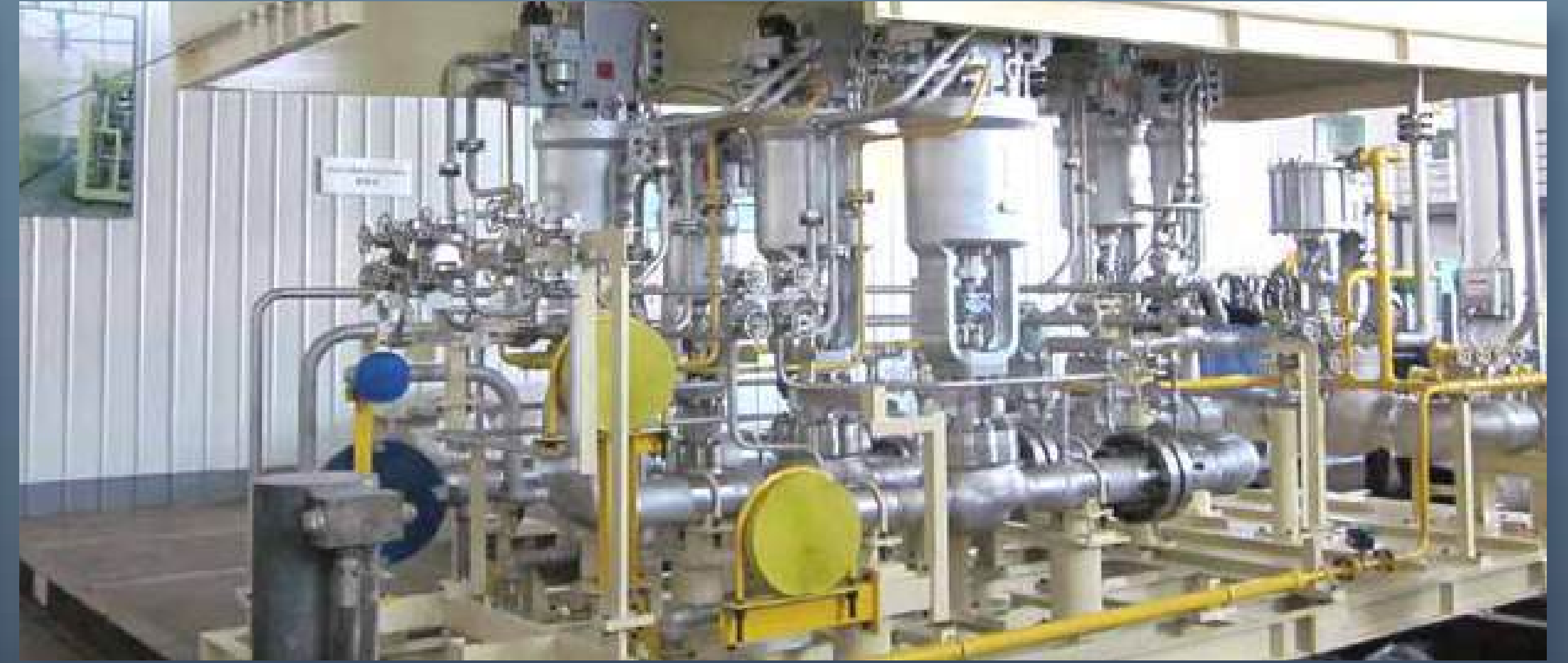
MITSUBISHI POWER FUEL GAS SKID
